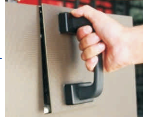
step 3 Pull the tool gently, Taking off the module
