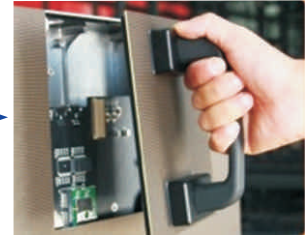
step 4 Replace a new module in the same way
