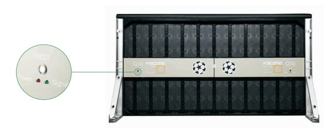
This function makes trouble-shooting process more efficient and easier, which can also detect the unusual operation of the display timely.
